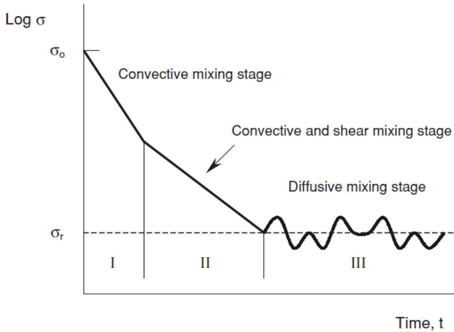
Figure 2. Characteristic curve of mixing process (adapted from Miyanami, 1997).
