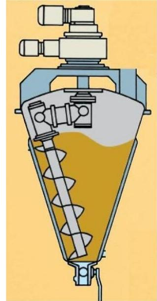
*Figure 4. Vertical conical mixer*
