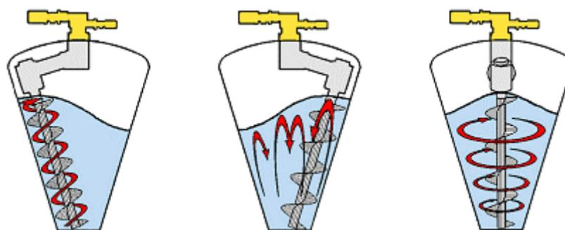
Figure 1. Different mixing processes in a vertical conical mixer
